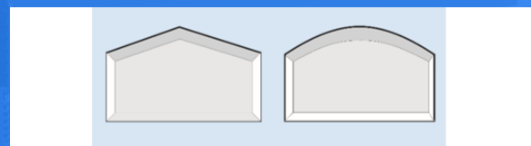
Figure G C. Simplifying Building Geometry for Energy Simulation Corresponding section: Building Envelope (Table G3.1, No. 5)—Different Tilt or Azimuth
