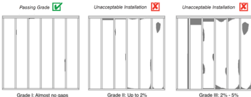
RESNET protocol for the effect of missing insulation on installation grade Diagrams from the HERS Standards
